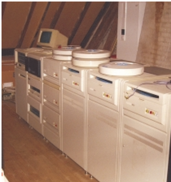
Fig. 9. DEC RL01 (on left) and RK07 (on right) Disk Drives (Courtesy Ákos Varga)
