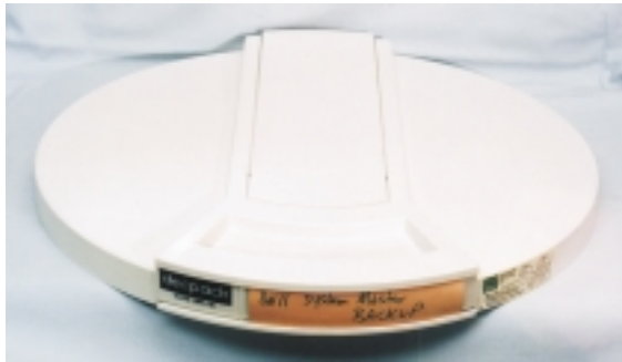
Fig. 10. DEC RK05 Disk Pack (Courtesy John Holden)
