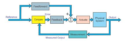
This section will discuss practical application of feedforward control to a feedback loop. In large part, feedforward can remove a lot of the potential error from the control loop, unburdening the feedback control system. But in some situations, it can introduce error. There are two basic forms of FF: Plant Injection (PI) and Closed Loop Injection (CLI).
