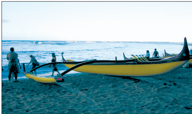
Figure 1. Outrigger canoes. The outrigger is an add-on mechanism that augments roll stability in a narrow-hulled boat such as a dugout. The operation of the outrigger is rather simple. When the canoe rotates so as to raise the boom from the water, the outrigger's weight at the end of a moment arm provides torque to rotate the boom back to the surface. When the rotation of the canoe pushes the boom into the water, the buoyancy of the boom restores the boom to the surface of the water.
