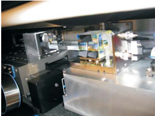
Fig. 6. Laboratory system: Aerotech air bearing linear stage, including linear grating for position measurement. The Aerotech system implements a PID controller and samples the data at 8 kHz. It has a built in swept-sine measurement. In the center of the image is a laser interferometer (IF) to provide an alternate measurement of the stage position. The stage itself is to the left of the IF.
