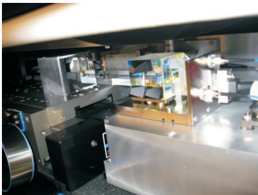
Fig. 10. Laboratory system: Aerotech air bearing linear stage, including linear grating for position measurement. The Aerotech system implements a PID controller and samples the data at 8 kHz. It has a built in swept-sine measurement. In the center of the image is a laser interferometer (IF) to provide an alternate measurement of the stage position. The stage itself is to the left of the IF.
