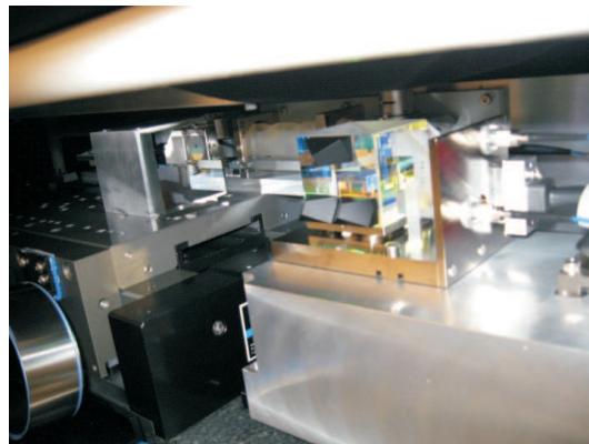
Figure 9.19: Laboratory system: Aerotech air bearing linear stage, including linear grating for position measurement. The Aerotech system implements a PID controller and samples the data at 8 kHz. It has a built in swept-sine measurement. In the center of the image is a laser interferometer (IF) to provide an alternate measurement of the stage position. The stage itself is to the left of the IF.
